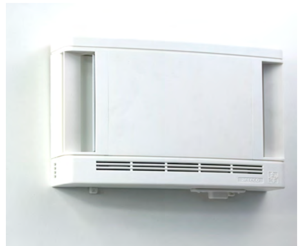
Components of a demand control ventilation system. A mechanical extract fan and wall vents react to humidity levels to increase the flow of fresh air to ensure good indoor air quality. Images courtesy Aereco Ltd
